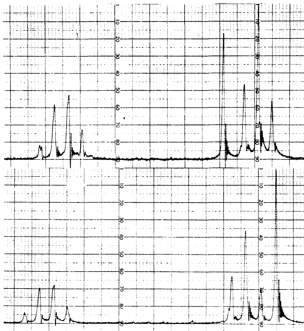
Fig. 2.—Nuclear magnetic resonance spectra: top, 2,2-dichlorocyclopropanone diethylacetal (IIb); bottom, cyclopropanone diethylacetal (XVIII).
